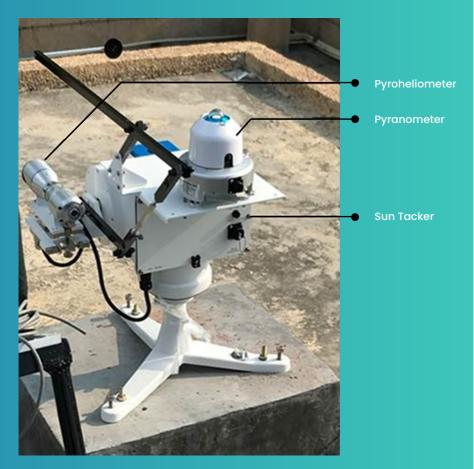
The Solar Monitoring Unit consists of a pyranometer and a pyrheliometer on a sun-tracking mechanical system.
