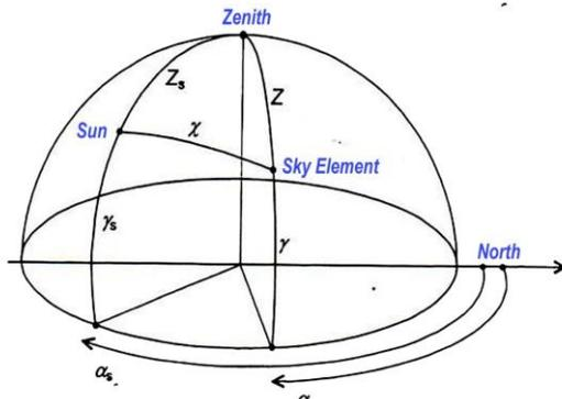
Alternatively, the angle of elevation,  $\gamma$ , may be used instead of the zenith angle,  $Z$ , to define the position of an element. (Refer Figure-3)
