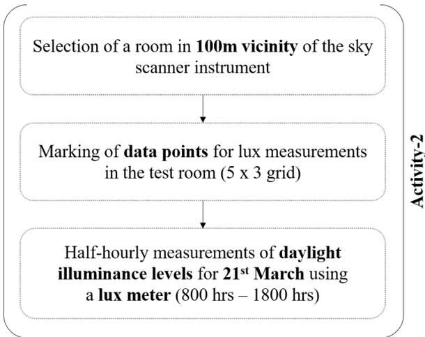
Figure 4. Daylight Illuminance Measurements
