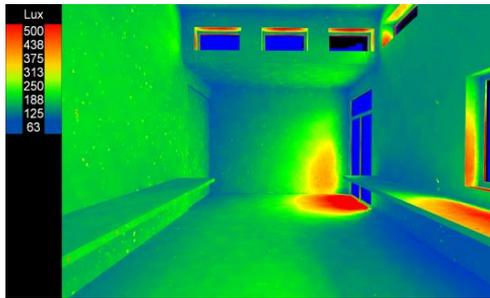
Figure 8. CIE Overcast Sky type daylight simulation for 21<sup>st</sup> March, 800 hrs with input sky type-1 described as ‘Overcast with a steep gradation and azimuthal uniform’
