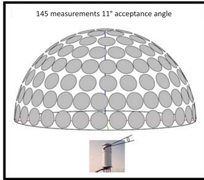
**Figure 3:** Representation of sky vault and number of patches studied by the Sky Scanner
