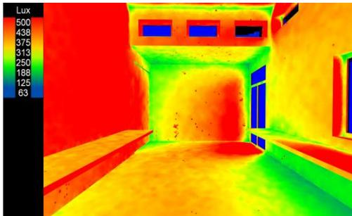
Figure 9. CIE Measured Sky type daylight simulation for 21<sup>st</sup> March, 800 hrs with input sky type-12 (see Table II) described as ‘Very clear/unturbid with a clear solar corona’
