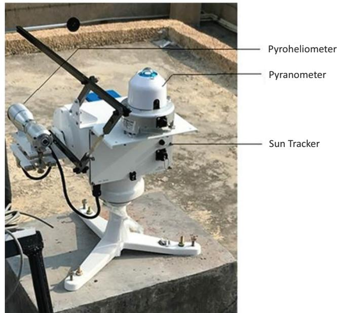
**Figure 5: Solar Monitoring Unit installed at the location Gurugram, India**
