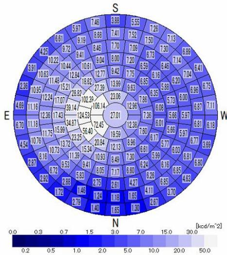
Figure 1. Measurement points for the sky scanner
