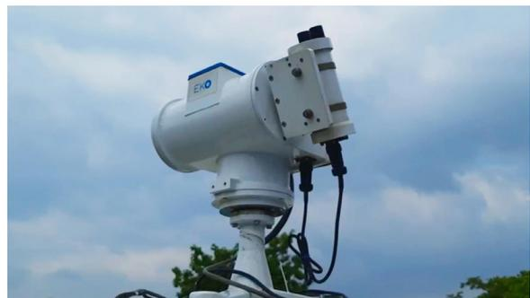
**Image 1:** Sky Scanner installed at the location Gurugram, India
