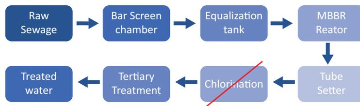
**FIGURE 40** Standard STP process excluding chlorination from contaminated water treatment
