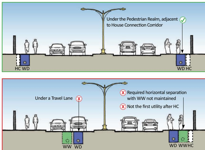
FIGURE 15 Typical potable water corridors' locations
