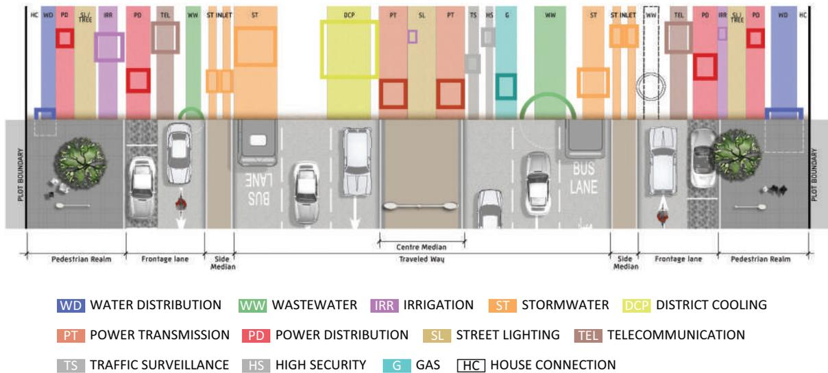
FIGURE 14 Typical utility corridor layout according to Utility Corridors Design Manual (UCDM)<sup>5</sup>
