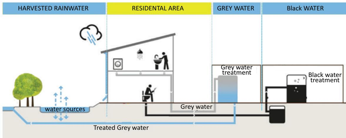
**FIGURE 38** Separate waste treatment plants installed at the facility to treat grey and black water separately
