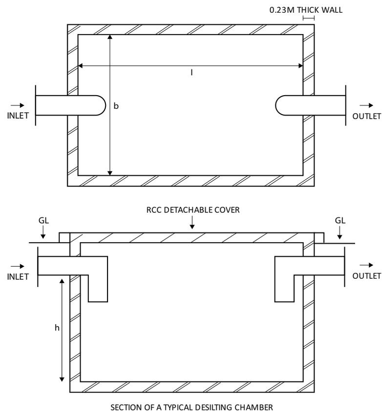
**FIGURE 48** Plan and section of a typical desilting chamber
