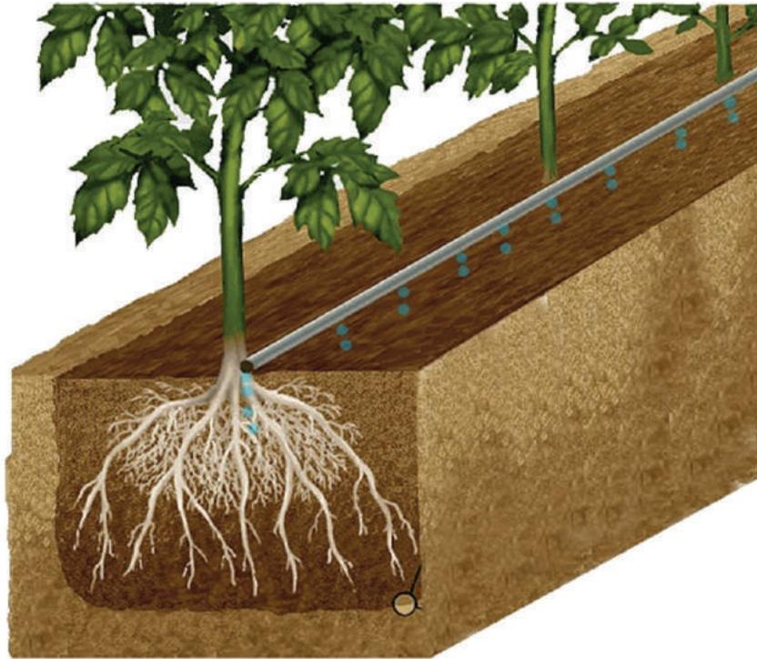
**FIGURE 31** A typical drip irrigation system being used for watering the plants
