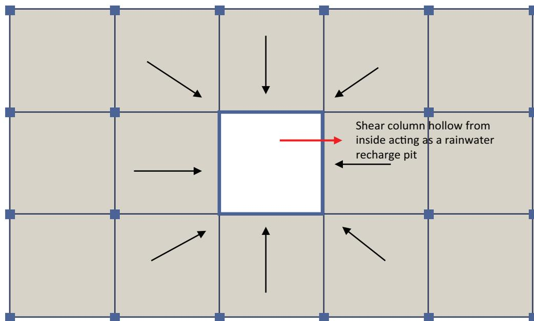
**FIGURE 46** Shear columns in basement acting as groundwater recharge structure
