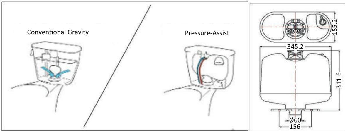
**FIGURE 8** Pressure-assisted versus conventional gravity-fed flushing system with plan details of pressure-assist tank
