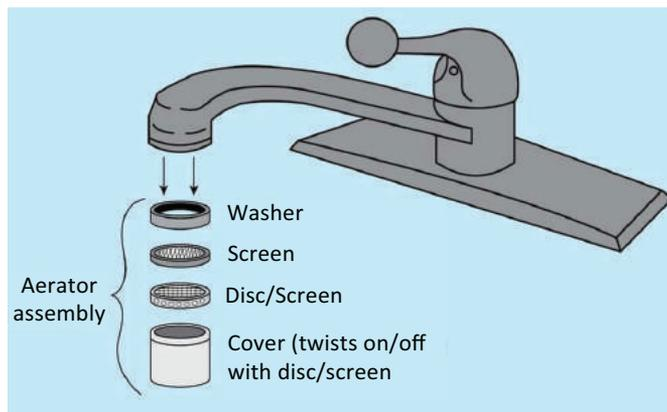
**FIGURE 9** A typical assembly of an aerator for sink water faucet
