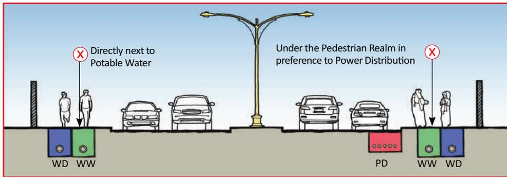
**FIGURE 16** Typical wastewater collection corridors' location
