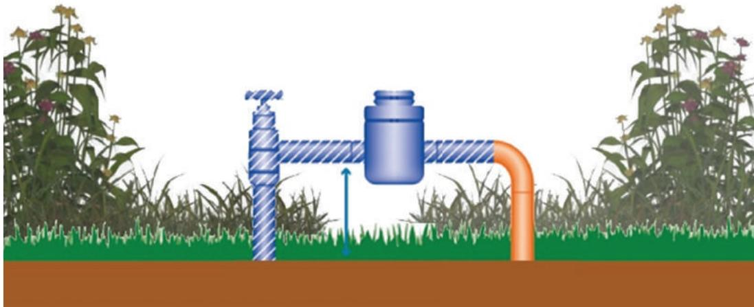
**FIGURE 34** Water meter installed to measure the amount of water being used for irrigating the plants
