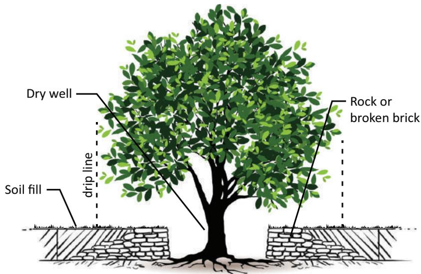
**FIGURE 25** Section of a dry well constructed to protect existing tree on site
