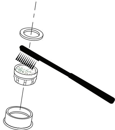
**FIGURE 24** Cleaning of a water faucet aerator using a brush
