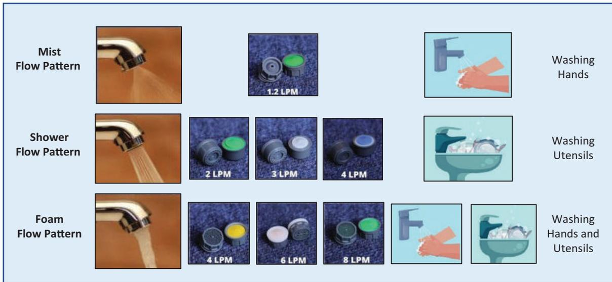
**FIGURE 10** Design types of water-saving aerators, their flow rates, and uses
