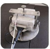
Thermal Constant Analyser rapidly and accurately measures the thermal conductivity, thermal diffusivity and specific heat capacity of a wide range of materials and encompasses high level of accuracy with material size flexibility.
