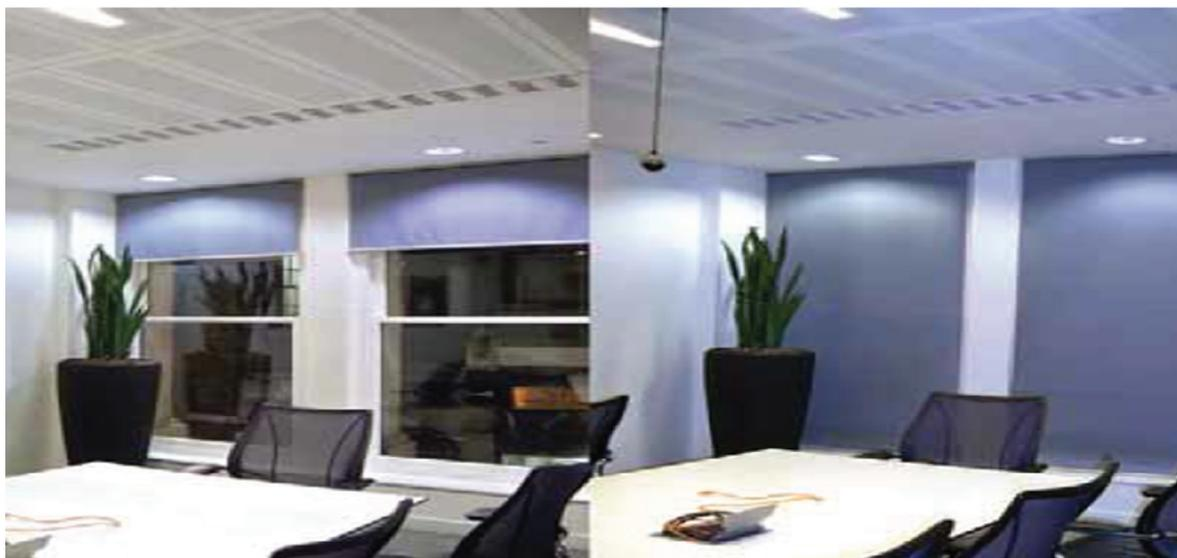
**FIGURE 6:** Comparison of the room with blinds raised and lowered showing the effect of changing the window wall reflectance
