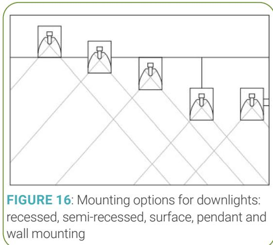
**FIGURE 16:** Mounting options for downlights: recessed, semi-recessed, surface, pendant and wall mounting
