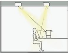
Luminaires placed on either side of the task (office desk) should not be directly above the observer.
