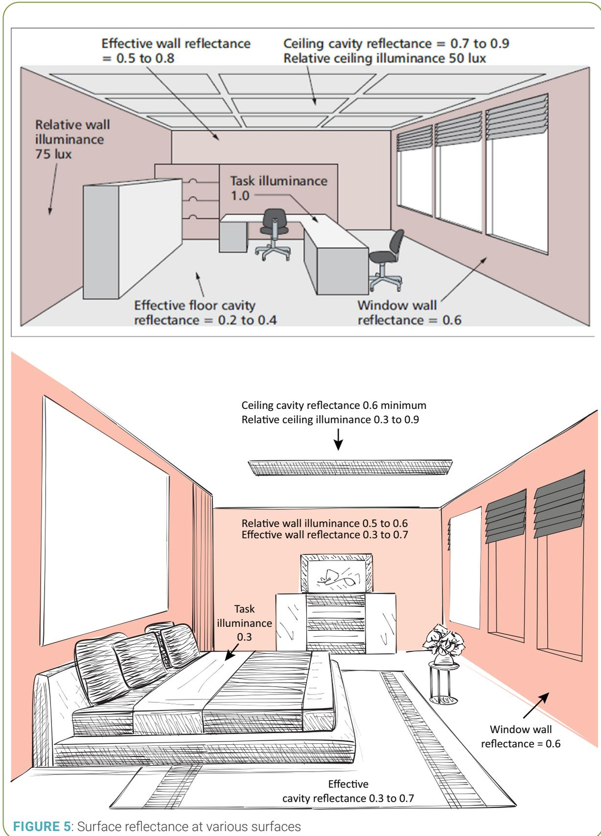
FIGURE 5: Surface reflectance at various surfaces
