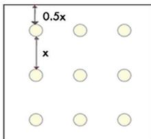
In general, luminaires are spaced  $x$  metre apart in either direction, while the distance of the end luminaire from the wall is  $0.5x$  metre. The distance  $x$  is more or less equal to the mounting height  $H_m$  between the luminaire and the working plane
