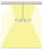
A direct/indirect pendant is a ceiling-mounted lighting fixture that directs the light upwards and downwards simultaneously. These types of fixtures thus provide a combination of general lighting and task lighting, and are widely used in offices and commercial spaces. These fixtures are designed in variations to enable designers with control over the light distribution up and down as per the requirements.
