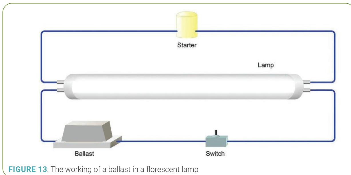
**FIGURE 13:** The working of a ballast in a florescent lamp
