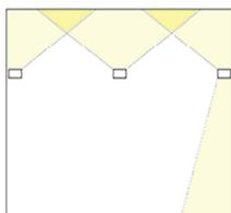
Indirect lighting, or up lighting, can create a low glare environment by uniformly lighting the ceiling (e.g. cove-type fixtures, lighted valences, wall washers, floor lamps). Use it wherever possible to produce high levels of ambient light
