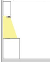
Under cabinets lights are task-specific lighting. These lights are often mounted below cabinets/shelves so that the objects on the counter below can be seen easily. These can be found in kitchen, accessory showcase, etc. in homes and in offices. They are generally controlled from a nearby switch or a switch on the light fixture.
