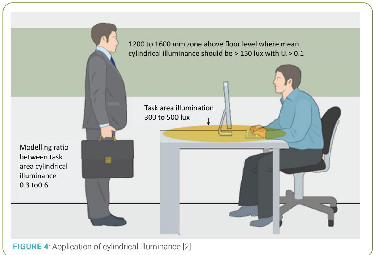
FIGURE 4: Application of cylindrical illuminance [2]
