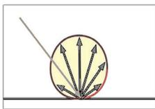
Use proper or correct lighting and avoid specular materials such as metallic paint on mechanics or wall rock, and choose flat paint when possible (surface reflectance)
