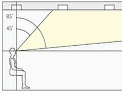
Local/task lighting should not be installed in the forbidden angle (field of vision) as it will become a source of direct glare (with respect to the height of lighting installation) or mount luminaires out of the field of view of the common workplace.
