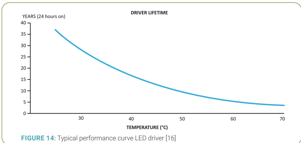
**FIGURE 14:** Typical performance curve LED driver [16]
