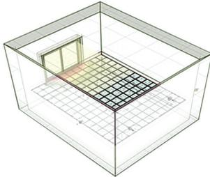
In-office buildings windows of height, 1.2 m or more in the centre of a bay with sill level at 1.0 to 1.2 m above the floor and in residential buildings windows of height 1.0 m to 1.1 m with sill height as 0.7 m to 0.9 m above the floor are recommended for good distribution of daylight indoors. Window width can accordingly be adjusted depending upon the required fenestration percentage of the floor area.
