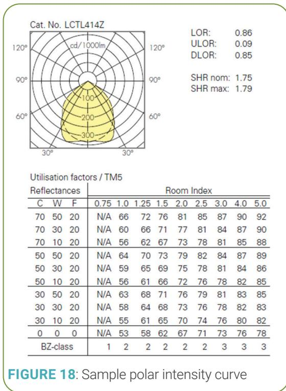
FIGURE 18: Sample polar intensity curve
