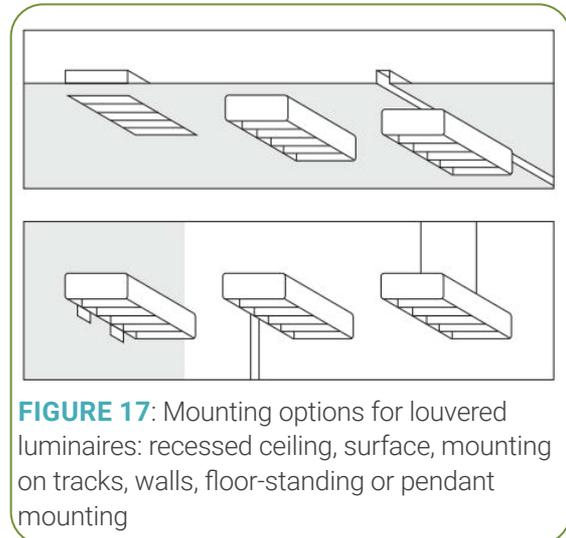
**FIGURE 17:** Mounting options for louvered luminaires: recessed ceiling, surface, mounting on tracks, walls, floor-standing or pendant mounting
