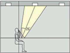
To evaluate direct glare, the luminance of the luminaires within the range 45° to 85° is considered.
