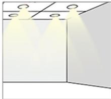
For small rooms where the room index<sup>1</sup> ( $K$ ) is less than 1, the distance  $x$  should always be less than  $H_m$ , as otherwise luminaires cannot be properly located.
