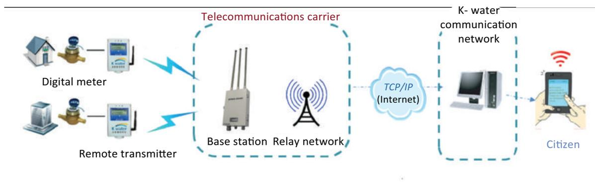
**FIGURE 12** Outline of smart metering system in Seosan city<sup>2</sup>
