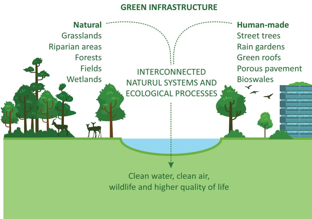
**FIGURE 43** Components of green infrastructure<sup>1</sup>
