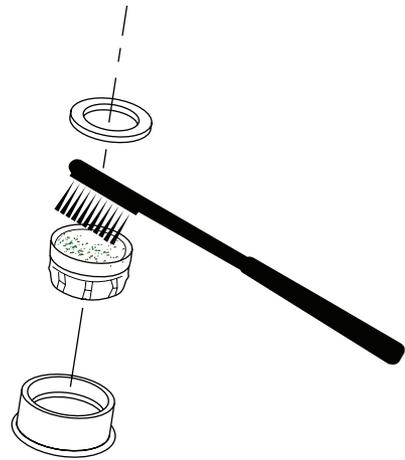
**FIGURE 24** Cleaning of a water faucet aerator using a brush
