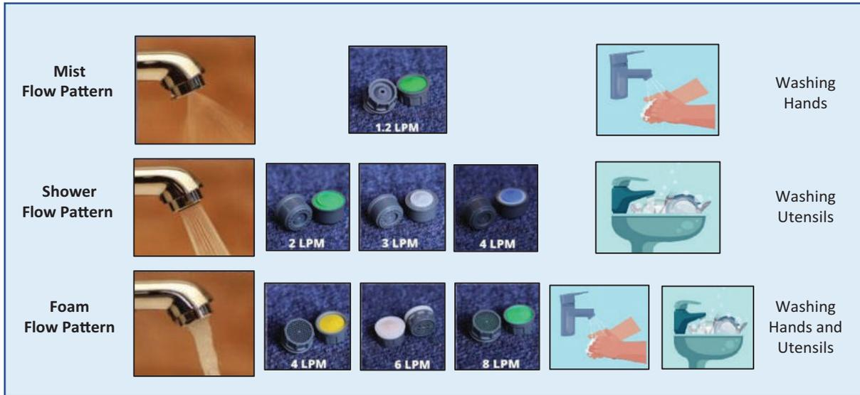
**FIGURE 10** Design types of water-saving aerators, their flow rates, and uses
