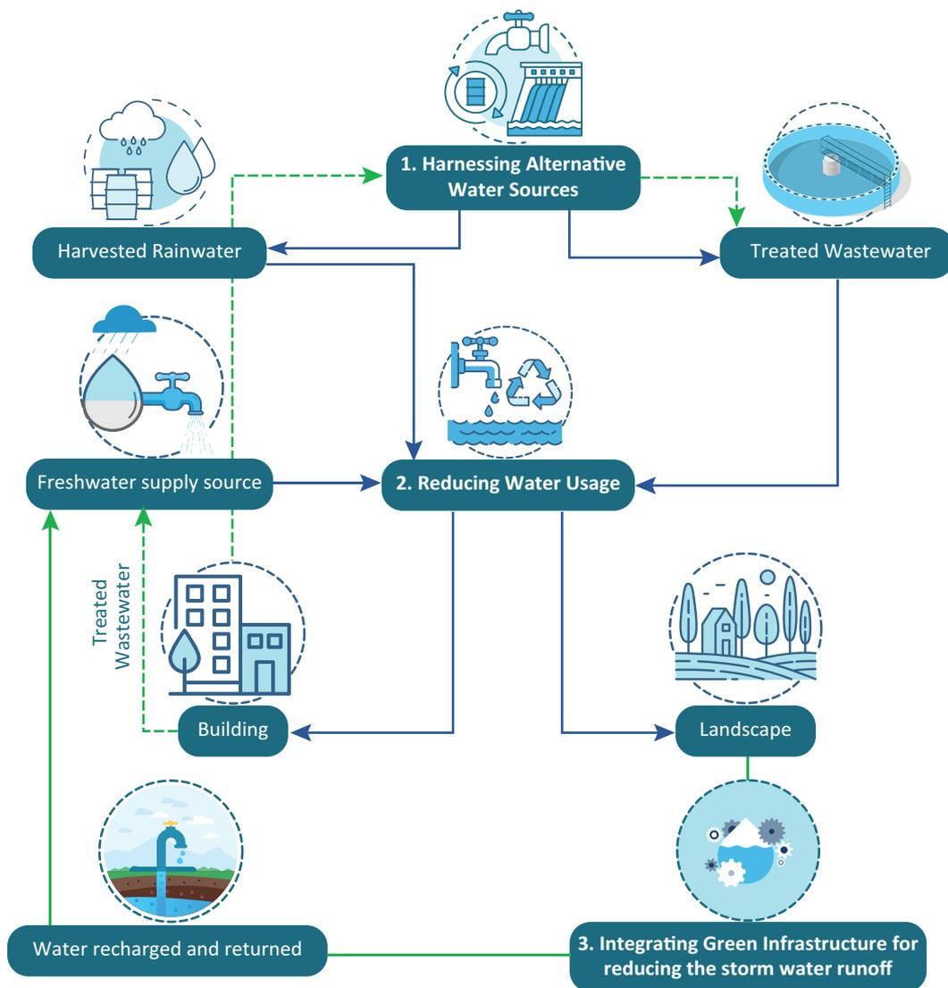
**FIGURE 5** The three-point approach for achieving water efficiency in a residential township
