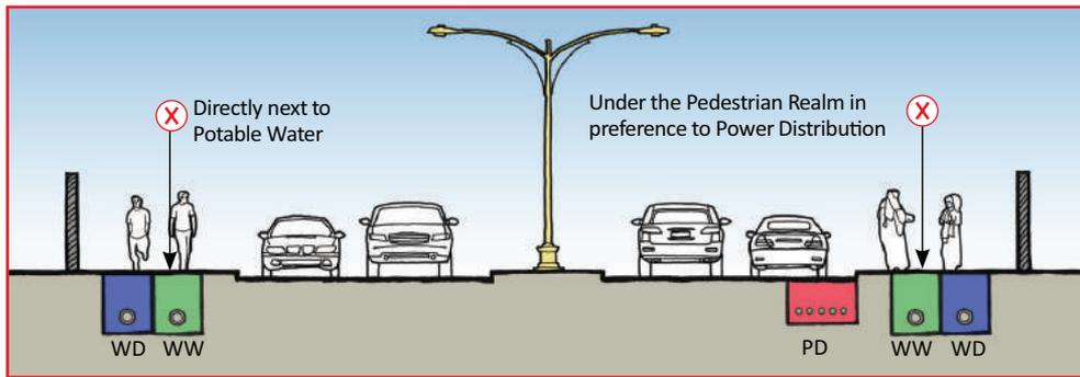
**FIGURE 16** Typical wastewater collection corridors' location
