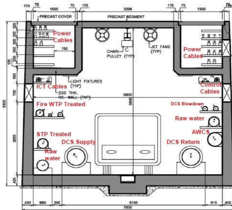
FIGURE 21 Utility tunnel, showing dimensions
